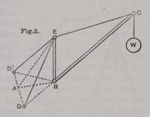
determines S', the pull on this stay. But it is clear that S' must be the resultant pull on the two original stays, and may be considered as a force applied at E in the direction of AE to the simple triangular frame DED'. A second diagram of forces therefore will determine the pull on each stay, just as in the next following case.
