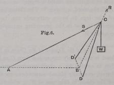
often of great length, resting on the ground at DD' and united at C, so as to be capable of turning together about DD' as an axis. The load is carried at C and the legs are supported by a stay, CA,
