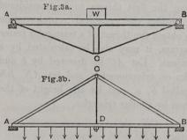
now a weight, W, be placed at the centre, immediately over the strut, it does not bend the beam (sensibly) as it would do if there were no strut, but is transmitted by the strut to the joint C, so that the truss is equivalent the simple triangular frame of the last article. This, however, supposes that
