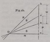
difference in the diagrams being that in the present case AC, which is now a tie, is divided into two parts, AE and EC, inclined at an angle. The stress on AE is therefore not the same as on EC, but is got by drawing a third line, Oa', parallel to AE. The perpendicular On gives us in this instance not only the stress on AB and the horizontal thrust
