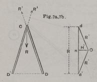
the triangle CDD', as in Fig. 7a, and imagine it loaded at C with a weight, R, then drawing the diagram of forces, Fig. 7b, we get R' the thrust on each leg. The horizontal force, H', in this second diagram represents the tendency of the feet of the legs to spread outwards laterally, while the force, H, of the original diagram represents their tendency to move in-
