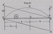
first the simple case of a beam of span l, supported at the ends and suppose a single concentrated load W to travel across it in the direction of the arrow. Let us consider any point K (Fig. 38) in the beam, distant a and b from the ends. As the load tra-
