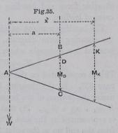
radiating lines AB, AC of a line drawn through the point parallel to the force. For example, the moment about  $K = M_K = Wx$ , where x is the perpendicular distance of K from the line of action of W.
