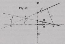
dropped from each intersection on to the line of action of the third force be r, p, q, respectively: by measurement on the drawing of the framework structure we are considering it is always easy to determine these perpendiculars. Then taking moments about the three points we get
