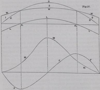
In the example the ship is supposed to be divided into any number of equal parts, and the weight of water displaced by each of those parts determined; ordinates are set up to represent those weights, and so, what is called a curve of buoyancy BBB (Fig. 37) is drawn. The whole area enclosed by the curve will represent the total buoyancy or displacement of the vessel, and is the same thing
