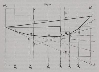
Commencing at O (Fig. 36), the point of application of P, draw any sloping line 0 1 2' cutting  $W_1$  in 1, and  $W_2$  in 2'. Then set up
