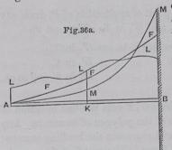
of expressing how the load is distributed is by means of a curve, the ordinate of which at any point represents the intensity of the load at that point. Such a curve is called a curve of loads. It may be regarded as the profile of the upper surface of a mass of earth or other material resting on the beam.
