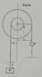
95. Verification of the Principle of Work in Special Examples.—We will now take some examples to illustrate and verify the principle of work, neglecting friction.
