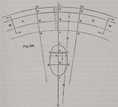
In the first instance the bending is supposed to be "simple," that is, it is not combined with shearing as is most often the case in practice, but is due to a uniform bending moment (see Art. 21). The curvature of the beam is then uniform, that is to say, it is bent into a circular arc. The investigation consists of three parts.
