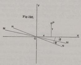
In Fig. 126 let MM be the axis of the bending moment, M inclined at an angle  $\theta$  to the principal axis of inertia GX, GY of the plane section. Then the couple M may be resolved into two components  $M\cos\theta$  and  $M\sin\theta$ , each of which will produce stress at any point
