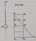
146) the tension of the string pulling upwards, being represented by BN, will be less than W acting downwards. Moreover, in the descent  $B_0B_1$  an amount of energy has been exerted by the weight represented by the area of the rectangle  $B_0M_0MB$ .
