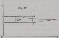
difference of pressure ΔP is represented by the difference ab of a pair of ordinates. The original volume of the air is represented by a1. Suppose now that in flowing through a passage of any description the air is heated, as for example x in passing through a furnace,
