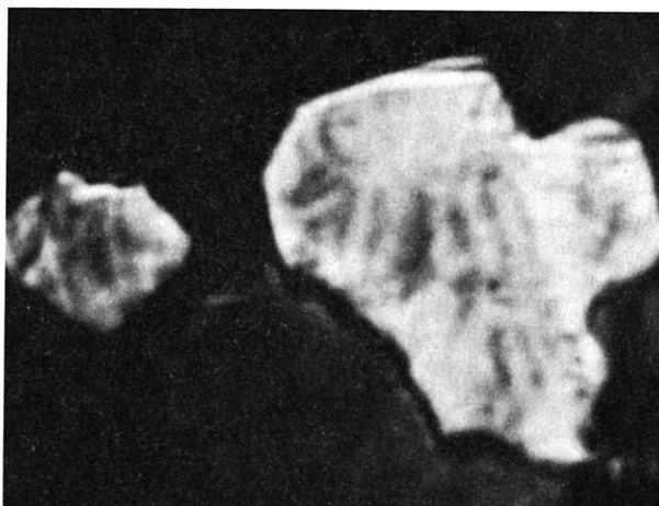
Fig. 4: Domain configuration of two titanomagnetite grains in the Parkstein basalt (Bitter pattern technique). For the scale see Fig. 5. Ambient field is zero.
