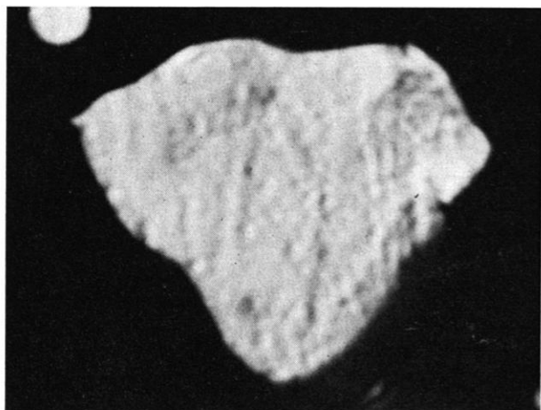
Fig. 6: Titanomagnetite grain in the Raue Kulm basalt, polished by ionic bombardment. The pits are dislocation lines intersecting the surface and inclusions. The thin straight lines are former scratches produced by previous mechanical polishing. For the scale see Fig. 8.
