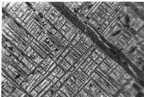
Fig. 8: An ore grain in sample No. 35. A complete pseudo-morphism of rutile (grey) and haematite (white) after ilmenite and exsolved titanomagnetite has taken place. The original exsolution structure is preserved. Magn.: 1200\times , oil immersion.
