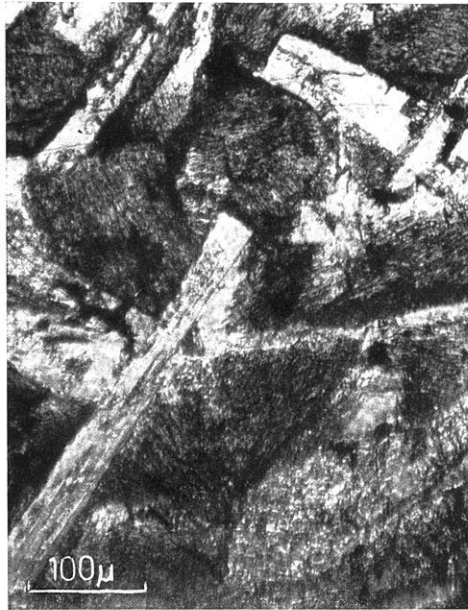
Fig. 6a. Photomicrograph (transmitted light, crossed polarizers) of a fresh sample (no. 63) from dyke-swarm showing primary igneous zonation in plagioclase (bottom) and primary augite (top); b Photomicrograph (transmitted light) of an incompletely metamorphosed sample (no. 118) from dyke swarm showing euhedral, compositionally zoned laths of primary plagioclase in a ground-mass of calcic amphibole (dark) and minor chlorite
