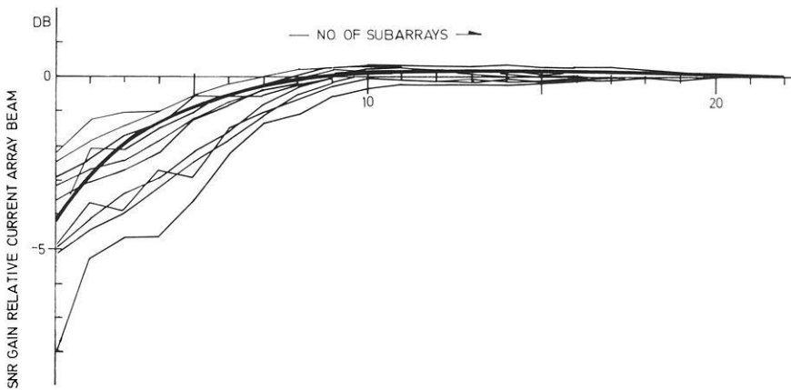
Fig. 8. Expected and obtained performance as a function of number of subarrays for DP beam no. 36. This beam is pointed towards 52N, 160E (off east coast of Kamchatka). The subarrays used have been ranked according to their amplitude. The first one is the one with the highest amplitude, in this case no. 3. The thick line shows the expected performance from the observed amplitude pattern, and corresponds to the dotted line on Figs. 5, 6 and 7. The thin lines give the observed values for 10 different events
