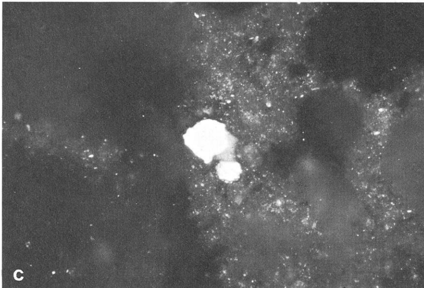
Fig. 4 a–c. Polished sections. The long side of the figures corresponds to 270 \mu\text{m} . a Pillow lava from site 12. Highly oxidized titanomagnetite grain with exsolved magnetite and ilmenite b Pillow lava from site 1/2. Hematite needles in the silicates c Radiolarite from site 30. Detrital magnetite grain and hematite needles
