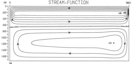
Fig. 1. Two layer convection,  $\Delta \rho/\rho = 10\%$ , temperature (contour interval 200°) and stream function (contour interval 20 dimensionless units). The chemical boundary is marked by dotted line. The spreading center is on the right, the subduction zone on the left
