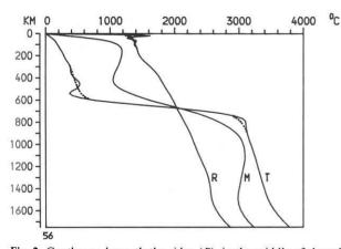
Fig. 2. Geotherms beneath the ridge (R), in the middle of the cells (M), and at the trench (T). Numerical over-swing effects are smoothed by *dotted lines*. The middle geotherm is representative for most of the length of the cell except narrow marginal regions
